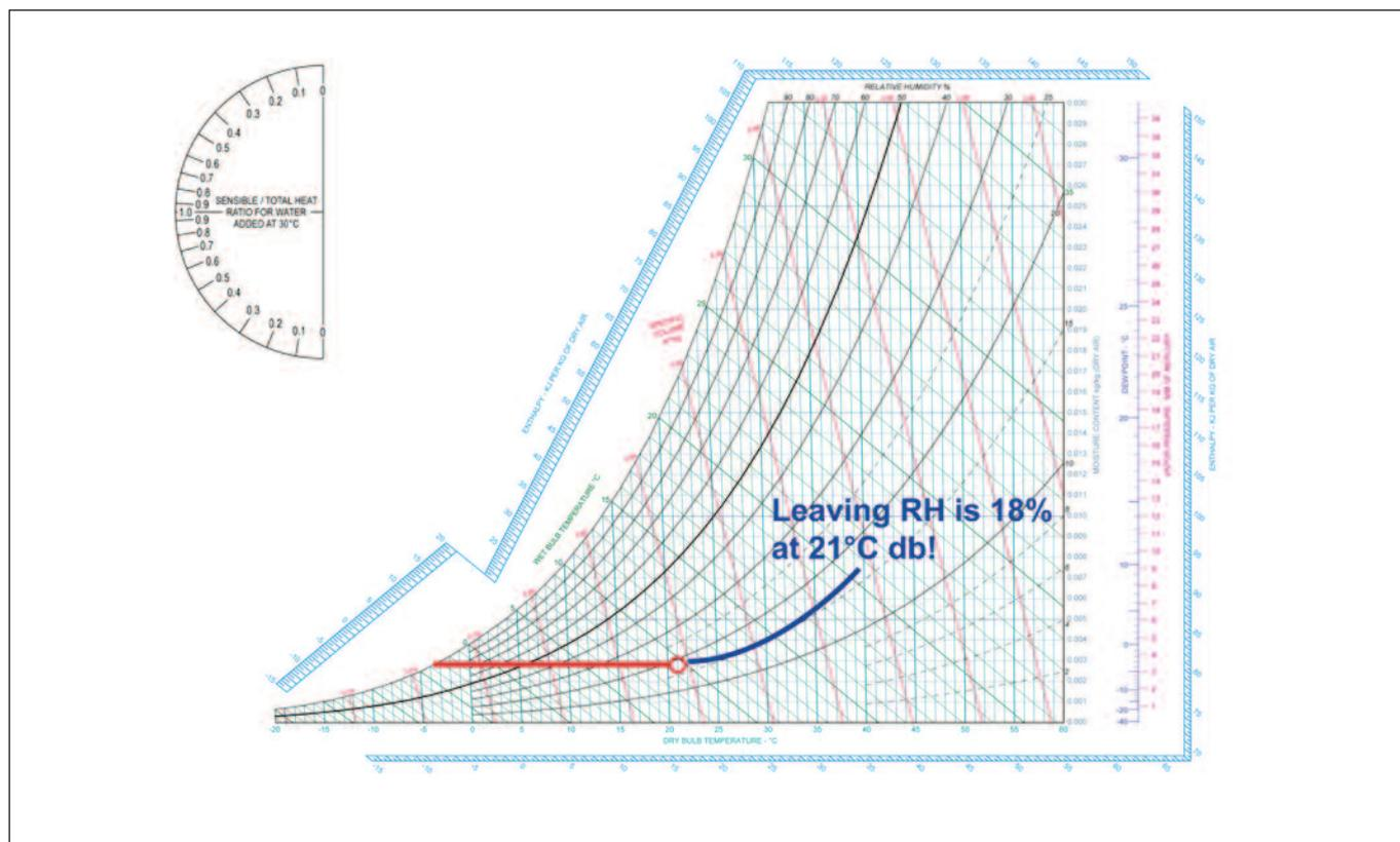
Figure 1: A psychrometric chart of a simple process – heating air, and the impact on RH.
