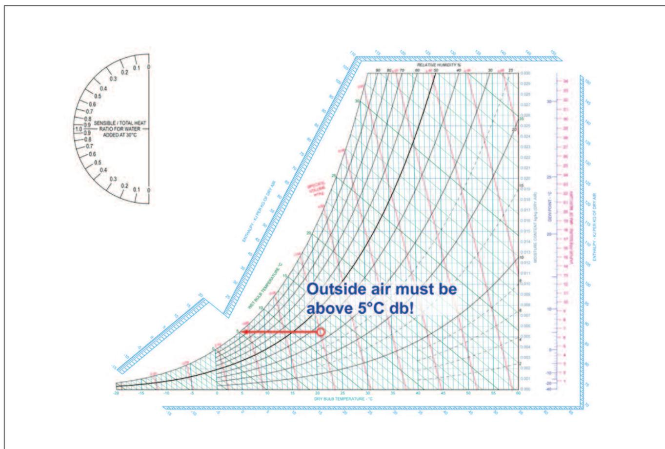
Figure 3: For a minimum 35% RH to be achieved without humidification, outdoor air would need to be above 5°Cdb.
